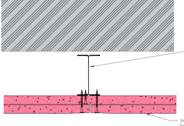
SPEEDLINE 70mm 'I' Studs at 600mm Ctrs
